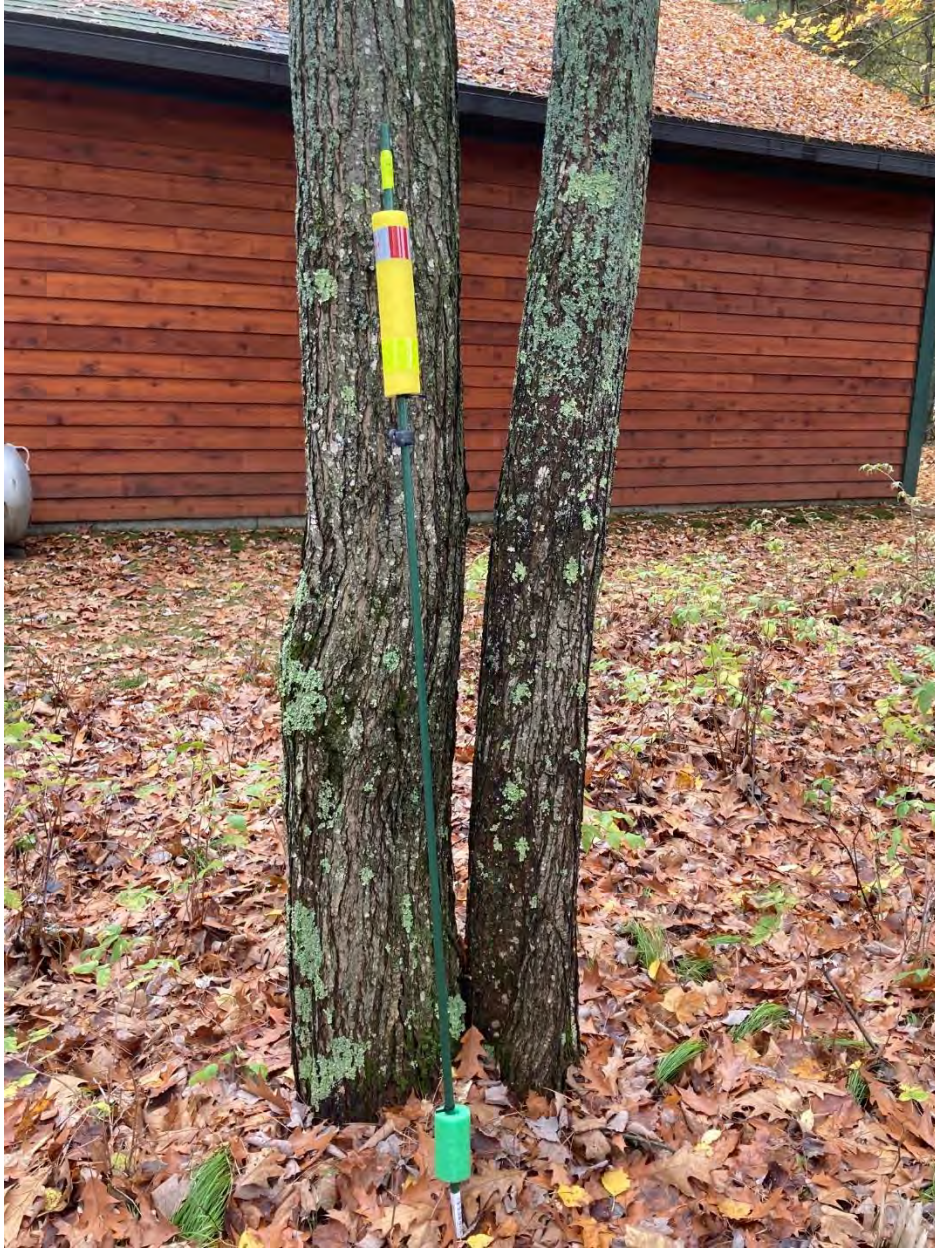
Barrier pole design. 6' pole with pool noodles on top and bottom, reflective tape, and rope holder (black piece below upper noodle). Zip ties were used to keep noodles in place.
