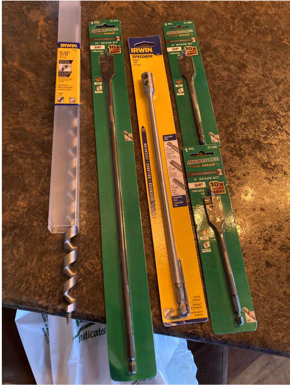
Bits and extension used to drill holes in ice to put up barrier poles.
